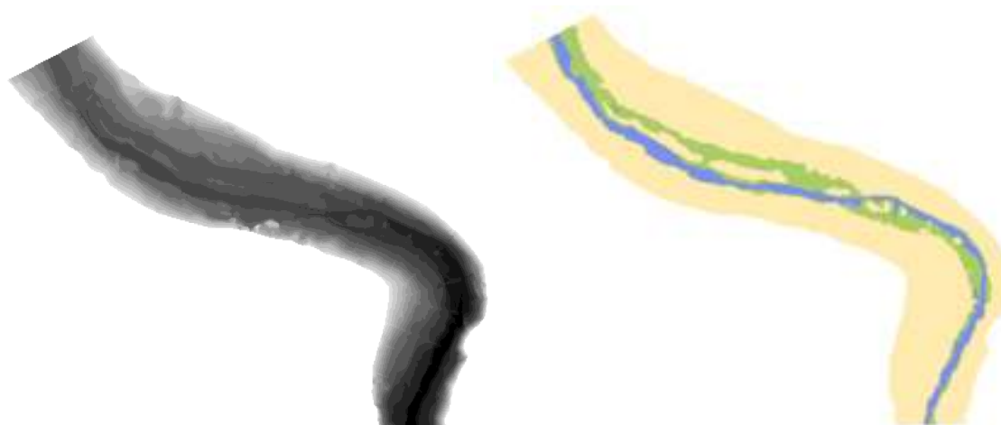
Figure 7.2. Digital elevation model (left) and hydrologic zones (right) including aquatic zone (blue), bank zone (green) and floodplain zone (yellow).
