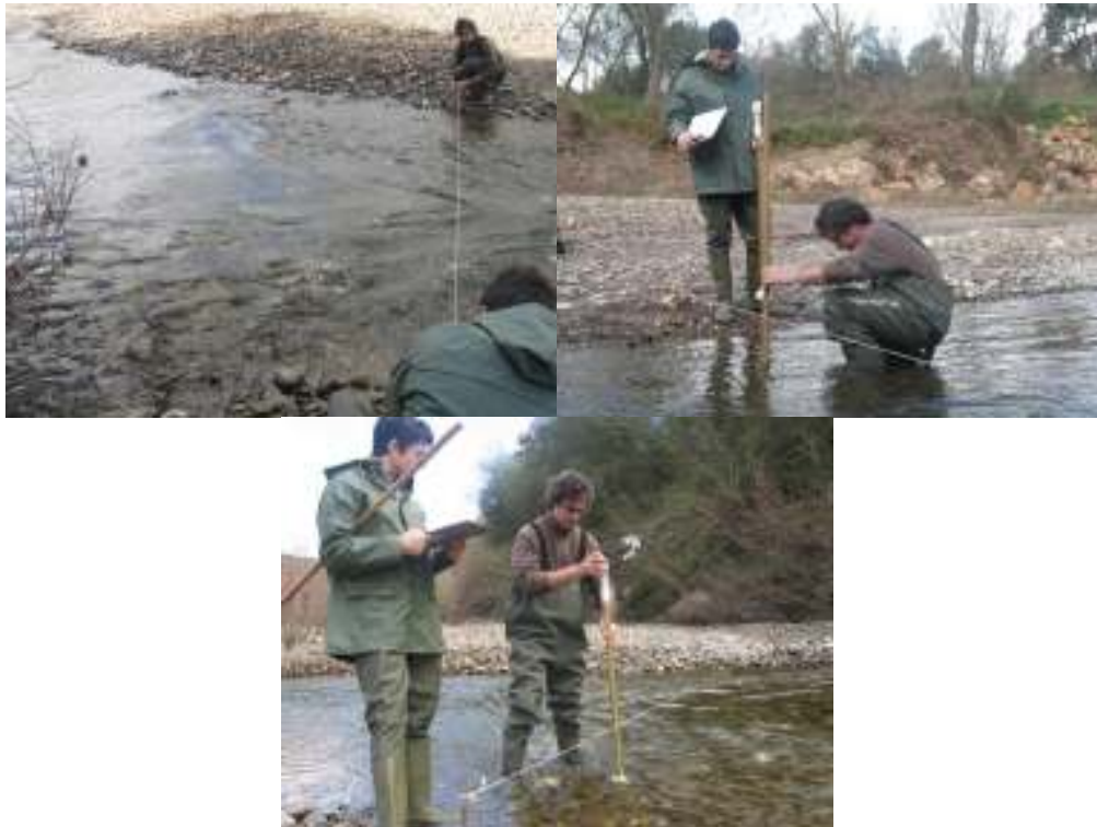
Figure 6.50. Flow estimation in a river section (from left to right and top to bottom, cross section signaling, water depth and velocity measurements).
