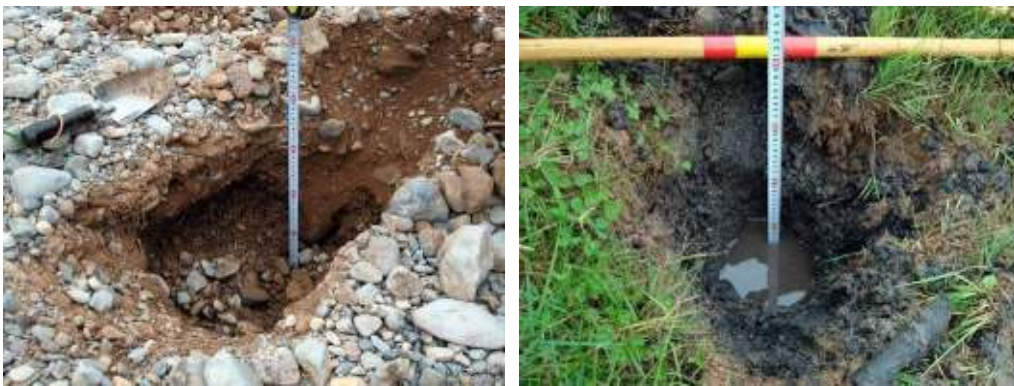
Figure 6.8. Example of soil sampling in the soil types 5 (left) and 8 (right).
