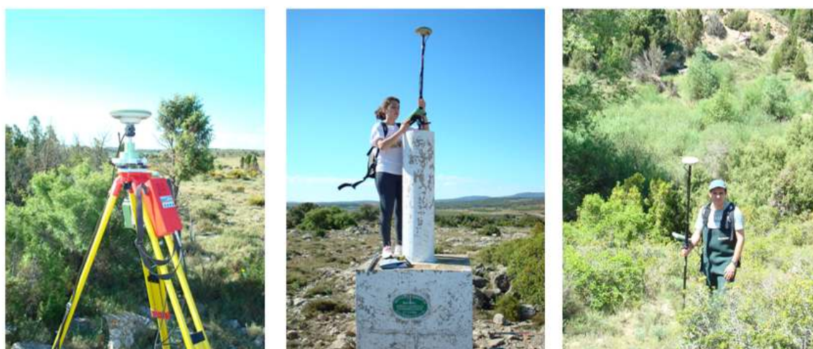
Figure 6.13. Assignment of absolute coordinates to the site. Fixed GPS unit (left) and mobile GPS unit in the Molino geodesic point (centre) and in the site Mijares-Terde (right).
