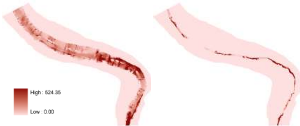
Figure 6.20. Shear stress (SS) for 40 m 3 /s (left) and 0.1 m 3 /s (right).
