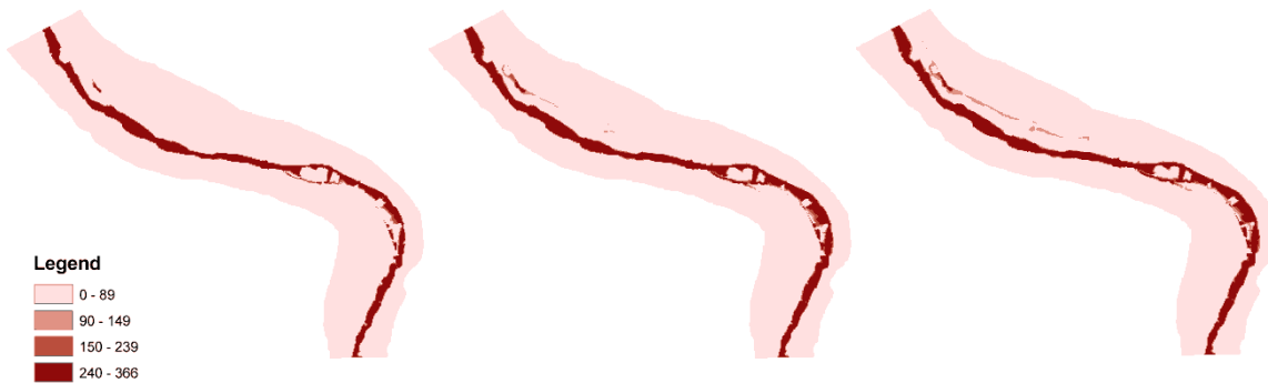
Figure 7.6. A selection of representative flood duration raster files corresponding from left to right, to medium, wet and very wet years (FD m , FD w and FD vw )
