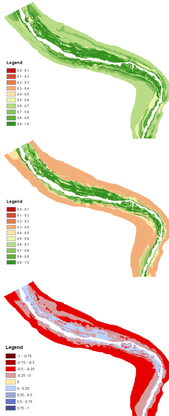
Figure 8.31. ETidx maps simulated for year 1980 in reference period scenario (above), for the equivalent year, 2090, in the HacCM3-PROMES (SRES A2) scenario (middle) and differences between them (below). Areas in red represent lower ETidx and areas in blue show higher ETidx values observed in the climate change scenario, in Terde reach (Spain)
